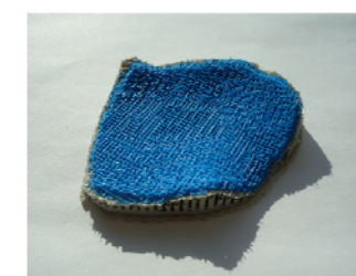
ABS scaffold with support structure.
