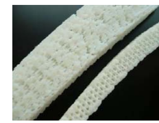
Partial printed 3D Cranial Implant.
